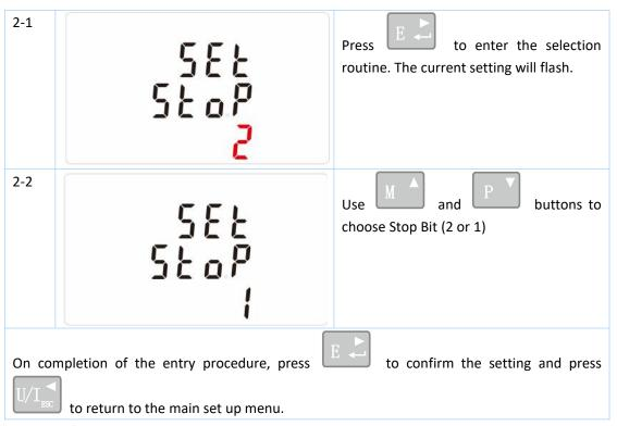
Note: Default is 1, and only when the parity is NONE that the stop bit can be changed to 2.
